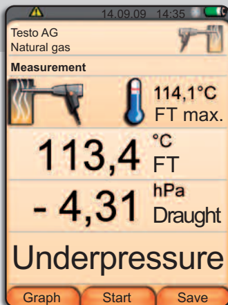
The result of the measurement: a negative pressure exists (-4.31 hPa)
