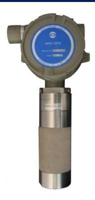
GasTech Australia Blind Guard series B-Guard<sup>TM</sup> Series GHD  $\mathrm{CO}_2$  detector is a single source dual wavelength instrument. The sensing and reference elements are self-compensating for optical integrity and other signal inhibitors. The industry standard 4 -20 mA analog output provides remote alarm, fault and calibration signals.
