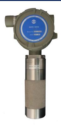
GasTech Australia Blind Guard series B-Guard<sup>TM</sup> Series GHD hydrocarbon detector is a single source dual wavelength instrument. The sensing and reference elements are self-compensating for optical integrity and other signal inhibitors. The industry standard 4 -20 mA analog output provides remote alarm, fault and calibration signals.
