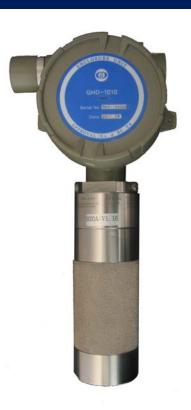
GasTech Australia Blind Guard series B-Guard<sup>™</sup> Series GHD hydrocarbon detector is a single source dual wavelength instrument. The sensing and reference elements are self-compensating for optical integrity and other signal inhibitors. The industry standard 4 -20 mA analog output provides remote alarm, fault and calibration signals.
