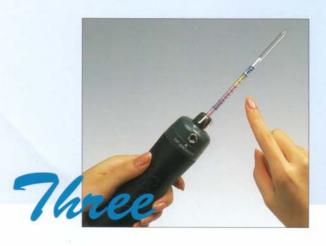
The color in the detector tube changes as the gas is drawn in. Wait the required sampling time and read the measurement at the end of the color changed layer. (Please note the concentration or mark the color changed demarcation on glass tube by a pen immediately).
