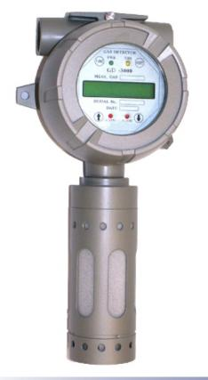
GasTech Australia Smart Guard series S-Guard™ Series GIR-3000 hydrocarbon detector is a single source dual wavelength instrument. The sensing and reference elements are self-compensating for optical integrity and other signal inhibitors. The industry standard 4 -20 mA analog output provides remote alarm, fault and calibration signals.
