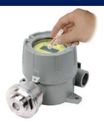
GasTech Australia Smart Guard series S-Guard<sup>TM</sup> Series GTD-2000Tx hydrocarbon Gas detector is a Toxic gas and Oxygen smart transmitter. The electrochemical elements are self-compensating. The industry standard 4 -20 mA analog output provides remote alarm, fault and calibration signals.
