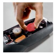
The sensor can be changed or upgraded in an additional gas parameter by the user directly on-site...
