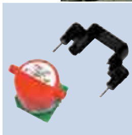
Gas sensor heating element – protects from damage caused by condensate and increases sensor reaction times when ambient temperatures are low
