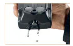
The measurement values can be read off on the well-lit display. The testo 310 has a battery life of 10 hours. It is excellently suited to rough surroundings. The condensation trap can be emptied quickly and easily.
