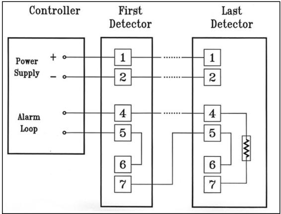
Figure 8. Typical Wiring Diagram for Four-Wire Controller
