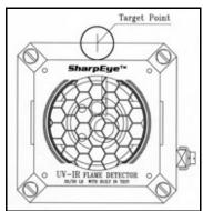
Figure 14: UV/IR Detector Target Point
