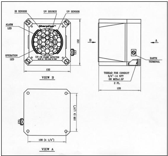
Figure 1. Flame Detector Assembly - Outline Drawing
