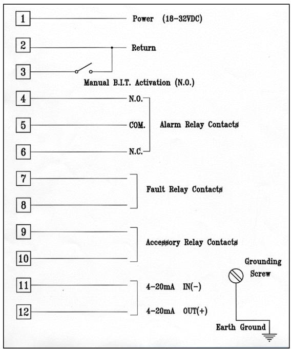
Figure 7. Flame Detector Assembly - Wiring Diagram
