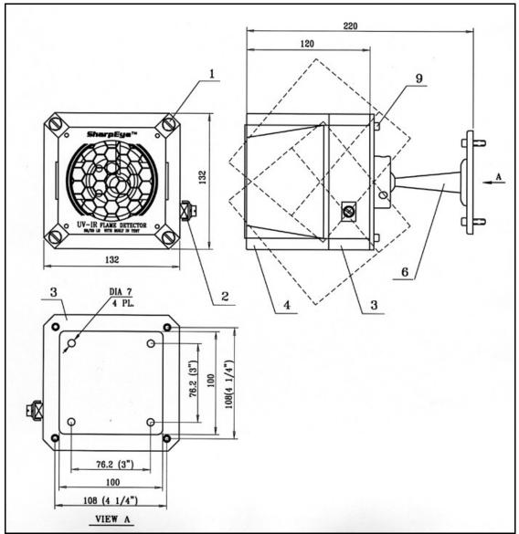
Figure 4.a. U/IR Detector and Swivel Mount Assembly
