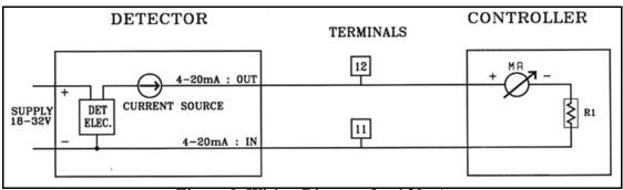
Figure 9. Wiring Diagram for 4-20mA
