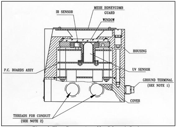
Figure 2. Flame Detector Assembly - Schematic Section
