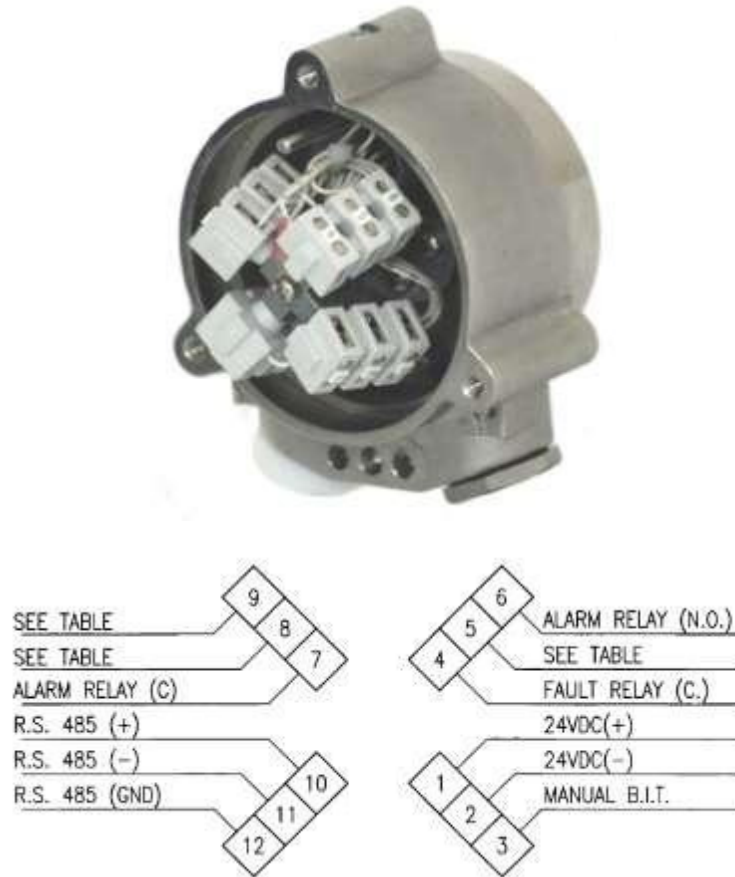
Figure 7: Wiring Terminals
