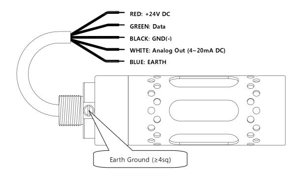
To supply the power to GSA920A, connect Red(+) and Black(-) from GSA920A to DC 24V terminal on the power supply and to receive analogue signal connect White from GSA920A to the analogue signal receiver device as above figure.
