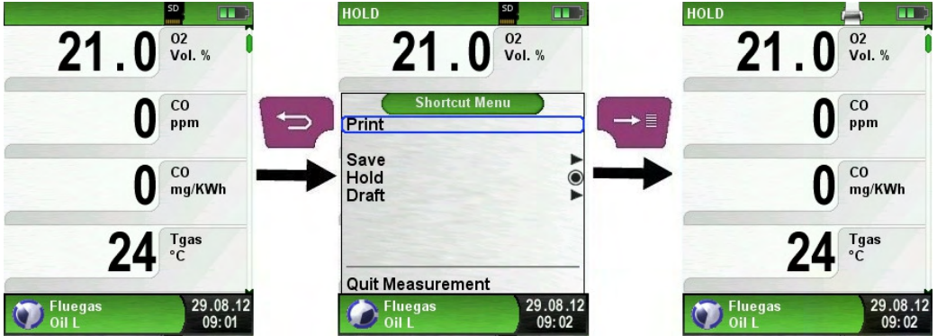
Fig 6: Direct access menu, (ex.: Flue gas measuring)
