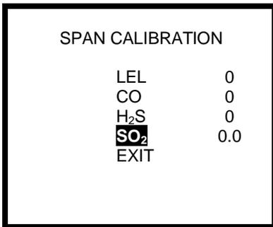
5. Use the up and down navigation arrows to highlight the sensor that requires calibration. Confirm the sensor selection by pressing the MODE button.
