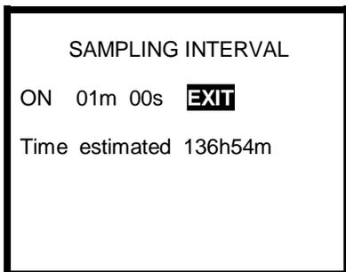
3. Use the navigation arrows to highlight the time interval (usually in minutes).
