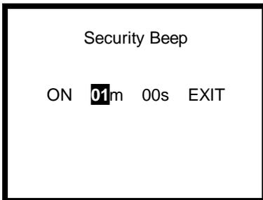
7. Once the desired interval is reached use the right and left navigation arrows to highlight EXIT.
