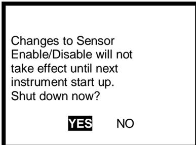
7. Click the MODE button with YES highlighted to shut the Cannonball3 down. Upon turn on the new sensor settings will go into effect.
