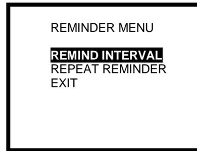
2. Use the navigation arrows to highlight "REMIND INTERVAL" and press the MODE button. The reminder interval will be shown as either "Every" with the number of days shown, or as "Never".
