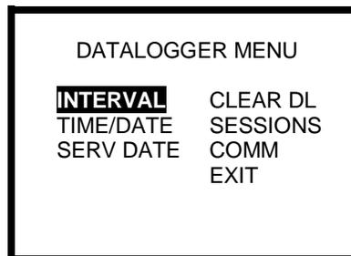
2. Use the navigation arrows to highlight INTERVAL and press the MODE button.
