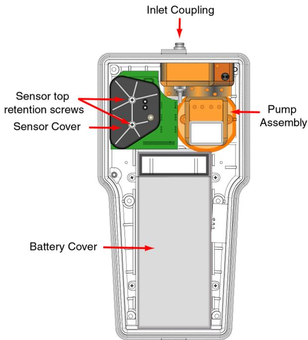
**Figure 6.1.1 Internal assembly diagram**
