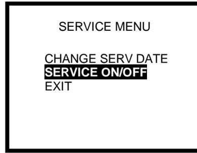
2. Use the up navigation arrows to highlight SERVICE ON/OFF and press the MODE button.
