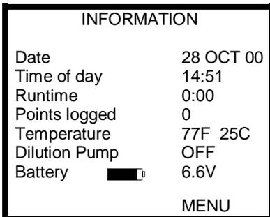
3. At the INFORMATION screen hold down the left navigation arrow for 3 seconds or until EXIT appears and is highlighted.
