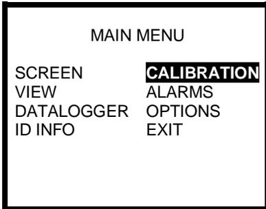
3. Use the navigation arrows to highlight CALIBRATION and press the MODE button.
