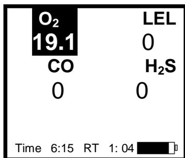
Current gas level screen in alarm condition in Basic, Basic/Peak and Technician Modes.
