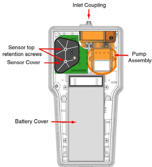
**Figure 2.6.3 Internal assembly diagram**
