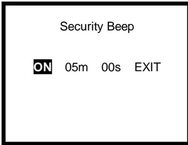
4. With ON or OFF highlighted, the up and down navigation arrows allow the user to toggle between security beep on and security beep off.
