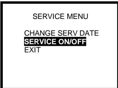
2. Use the up navigation arrows to highlight SERVICE ON/OFF and press the MODE button.
