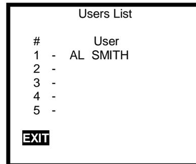
13. Press the MODE button with EXIT highlighted to exit the users list screen.
