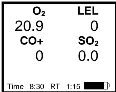
Current gas readings screens with CO Plus sensor; calibration gas value set to CO.
