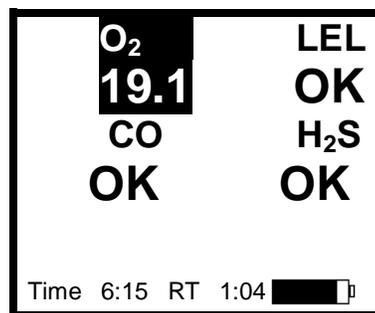
**Text Only mode current gas level screen with alarm condition.**
