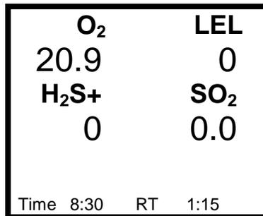
Current gas readings screens with CO Plus sensor; calibration gas setting set to H<sub>2</sub>S.
