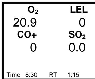
Current gas readings screens with CO Plus sensor; calibration gas setting set to CO.
