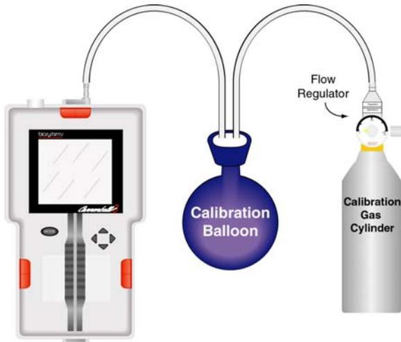
**Cannonball3 with calibration balloon and calibration gas cylinder.**
