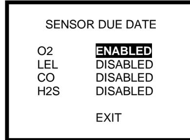
4. Once the sensor due date settings are enabled or disabled as required, press the MODE button to enter the settings.
