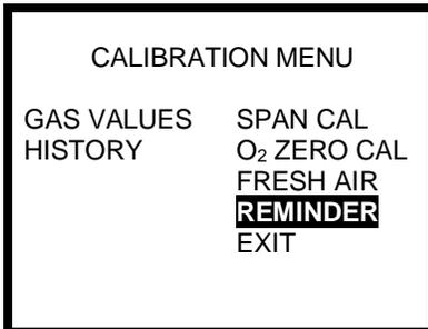
2. Use the navigation arrows to highlight REMINDER and press the MODE button to confirm the selection.
