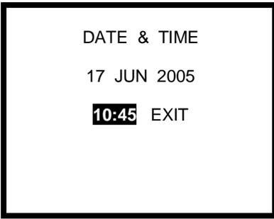
4. The MODE button may be pressed at any time to confirm the new time settings.
