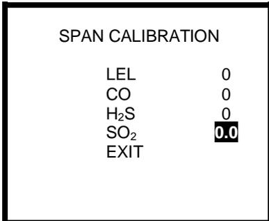
As discussed above, the Cannonball3 includes a built-in continuous sample draw pump that draws the gas sample into the sensor compartment. As such, there are two viable methods for delivering the gas to the sensor chamber for span calibration: a standard 1 liter/minute regulator with the calibration balloon that is included with every Cannonball3, or with a demand flow regulator and a small piece of tubing.
