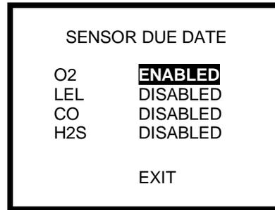
4. Once the sensor due date settings are enabled or disabled as required, press the MODE button to enter the settings.
