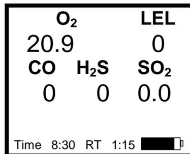
Current gas readings screen with Duo-Tox and SO<sub>2</sub> toxic sensors installed.
