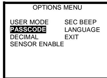
2. Use the navigation arrows to highlight PASSCODE and press the MODE button. The Passcode Menu will then be shown.
