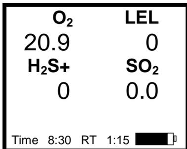
Current gas readings screens with CO Plus sensor; calibration gas value set to H<sub>2</sub>S.
