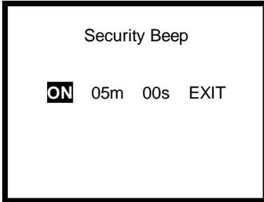
5. The interval setting will appear when the security beep is turned ON (as above). Use the right and left navigation arrows to highlight the interval if it requires adjustment.
