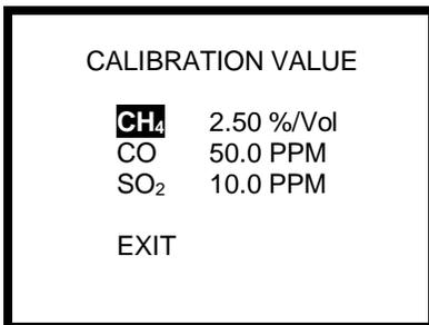
3. Use the up and down navigation arrows to select LEL or CH<sub>4</sub> and press the MODE button.
