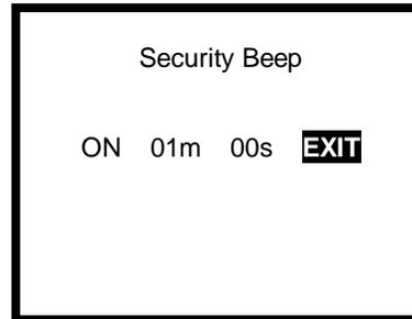
8. Press the MODE button with EXIT highlighted to exit the security beep option.
