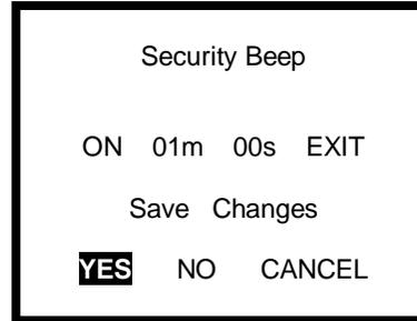
9. Press the MODE button with YES highlighted to save the new security beep settings.
