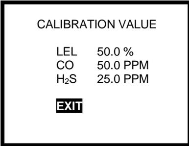
**⚠WARNING** Calibration values shown in the calibration value table must match those appearing on the calibration gas cylinder(s) that will be used to calibrate the Cannonball3. Non-matching calibration gas and calibration gas value settings will lead to inaccurate and potentially dangerous readings.
