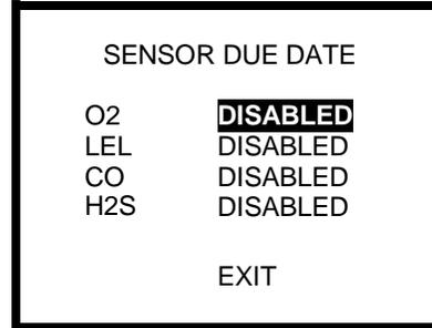
3. To change the service due setting for an individual sensor, use the up and down navigation arrows to highlight the setting adjacent to the sensor, the right or left navigation arrows may then be used to toggle back and forth between “enabled” and “disabled”.
