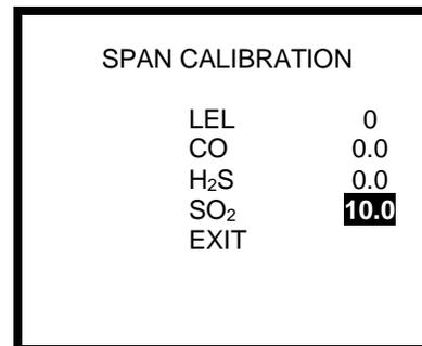
8. When the span calibration for a particular sensor is completed, press the MODE button to confirm the calibration and then use the navigation arrows to advance to the next sensor channel to be span adjusted. The sensor that was just span calibrated will then be marked with an arrow as shown below.
