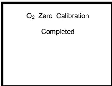
After the successful completion of the O<sub>2</sub> zero calibration, the instrument will return to the Main Menu. Disconnect the calibration gas cylinder immediately.
