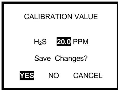
9. Press the MODE button with YES highlighted to save the new settings.
