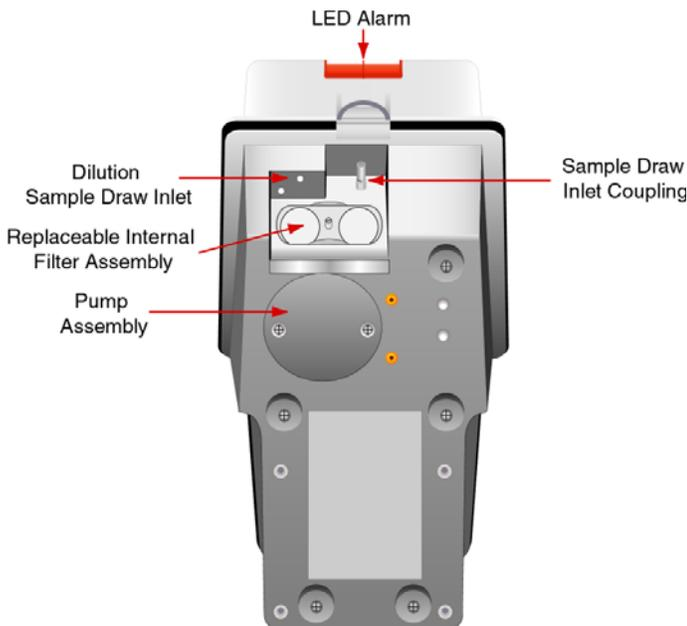
Figure 2.5.3 Bottom of lower case assembly.
