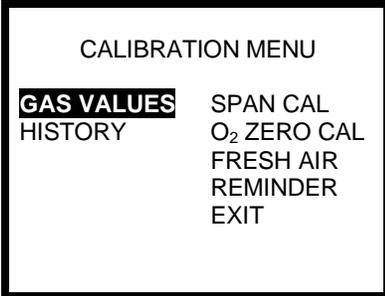
2. Use the navigation arrows to highlight GAS VALUES and press the MODE button.
