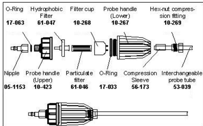
Figure 2.5.2. Cannonball3 sample draw probe.
