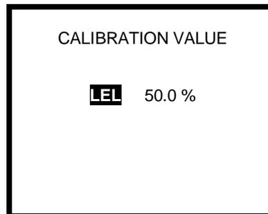
5. With LEL or CH<sub>4</sub> highlighted, the up and down navigation arrows are used to change the setting. Once the desired setting is shown, press the MODE button to save the setting or move on to step 6 to adjust the concentration of the calibration gas.
