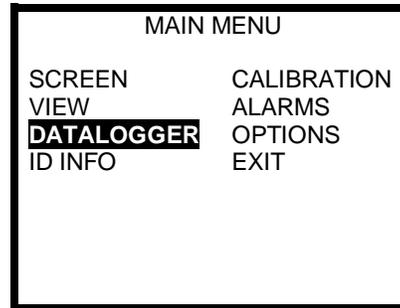
6. Use the navigation arrows to highlight DATALOGGER and press the MODE button.
