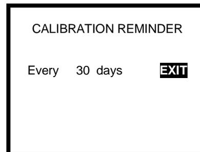
4. To enable or disable the Calibration Reminder, use the navigation arrows to highlight "Every" or "Never" and press the up navigation arrow to change it.
