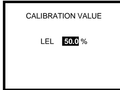
4. The right and left navigation arrows may be used to move back and forth between the calibration gas setting (LEL or CH<sub>4</sub>) and the calibration gas concentration. To change the calibration gas setting, press the left navigation arrow once to highlight LEL or CH<sub>4</sub>.
