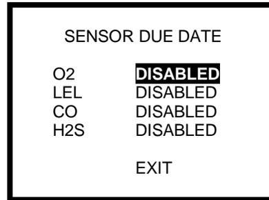
3. To enable (or disable) the service due setting for an individual sensor, use the up and down navigation arrows to highlight the setting adjacent to the sensor, and then press the right or left navigation arrow once.
