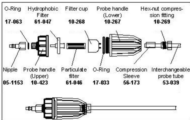
Figure 6.3 Cannonball3 sample draw probe.
