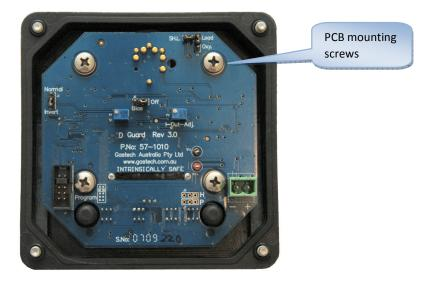
7. Gently remove the PCB which will expose the sensor.
