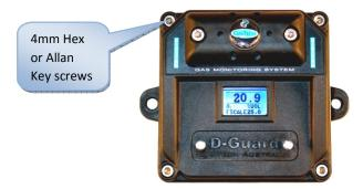
2. Gently remove the lid making sure that you don't lose the 4 lid screws or the large "O" ring that seals the lid to the base.
