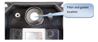
14. Fit new gasket and filter the same way as previously fitted. Use the sticky side to stick to the plastic enclosure.
