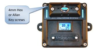
3. Gently remove the lid making sure that you don't lose the 4 lid screws or the Large "O" ring that seals the lid to the base.
