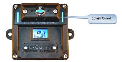
If the splash guard is fitted this will need to be removed so you can apply the gas directly to the sensor. Remove the splash guard by removing the two screws (4mm Alan key).
