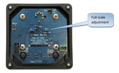
10. Once any adjustments have been made, remove the jumper between pins 1 and 2, screw the lid back together, close the calibration door and normal operation will resume.
