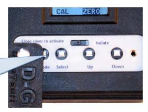
3. The first menu the D-Guard<sup>TM</sup> enters in calibration mode, is the zero menu. This mode is used during calibration, which will be discussed later in this section.
