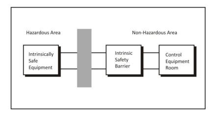
If you are utilizing the D-Guard<sup>TM</sup> in a Hazardous environment, you will need to select an appropriate IS barrier.
