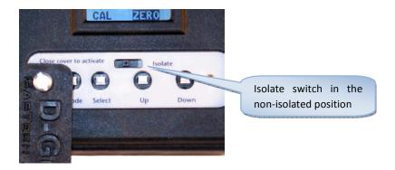
Flicking the Isolation switch over to "ISOLATE" will drop the mA signal down to 3mA and invert the display, the gas reading will flash, and the word "ISOLATED" is shown. This mode is permanent until the switch is changed over.
