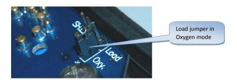
The table below shows the settings for the various GasTech oxygen sensors.
