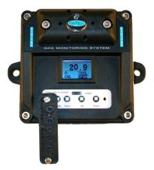
2. Once the calibration plate is removed, the mode button will be released sending the unit into calibration mode.
