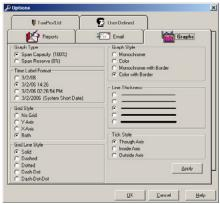
The Graph Type can be set to Span Capacity or Span Reserve, which controls the baseline placement (at either 0% or 100%) for the sensor span graph. The baseline represents the sensor's low capacity limit, which is an indicator of the relative health of the sensor.
