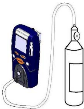
Figure 4.1 Bump Test / Gas calibration set up
