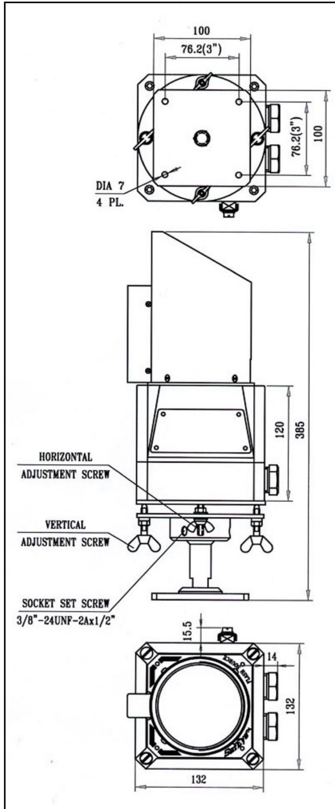
Figure 24. Source Outline Drawing (70 dia Lens Type) With Swivel Mount
