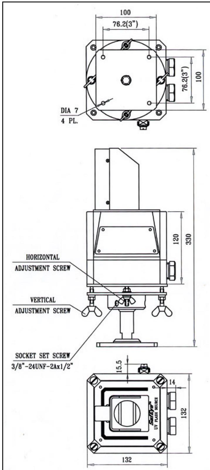
Figure 25. Source Outline Drawing (Reflector Type) With Swivel Mount
