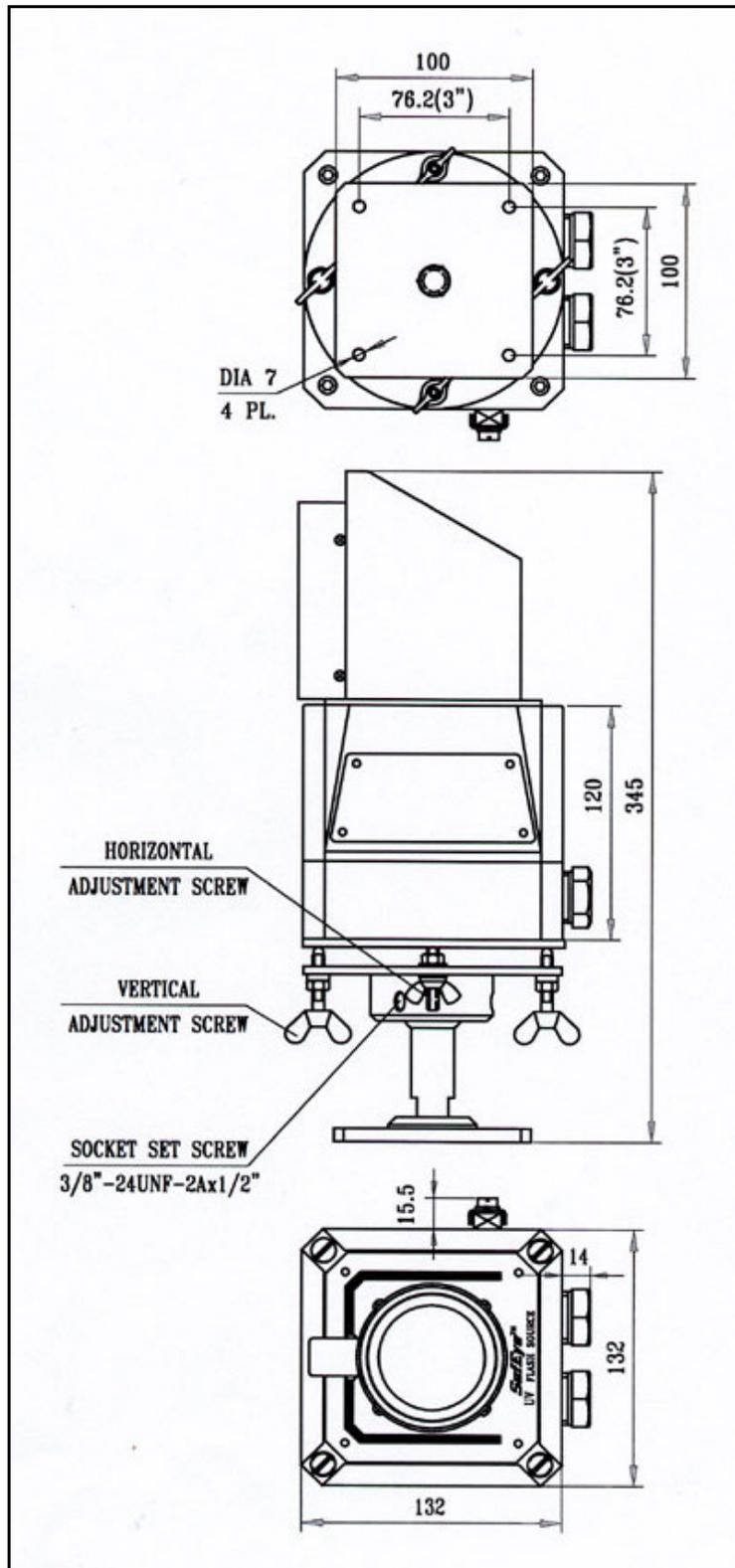
Figure 23. Source Outline Drawing (40 dia Lens Type) With Swivel Mount
