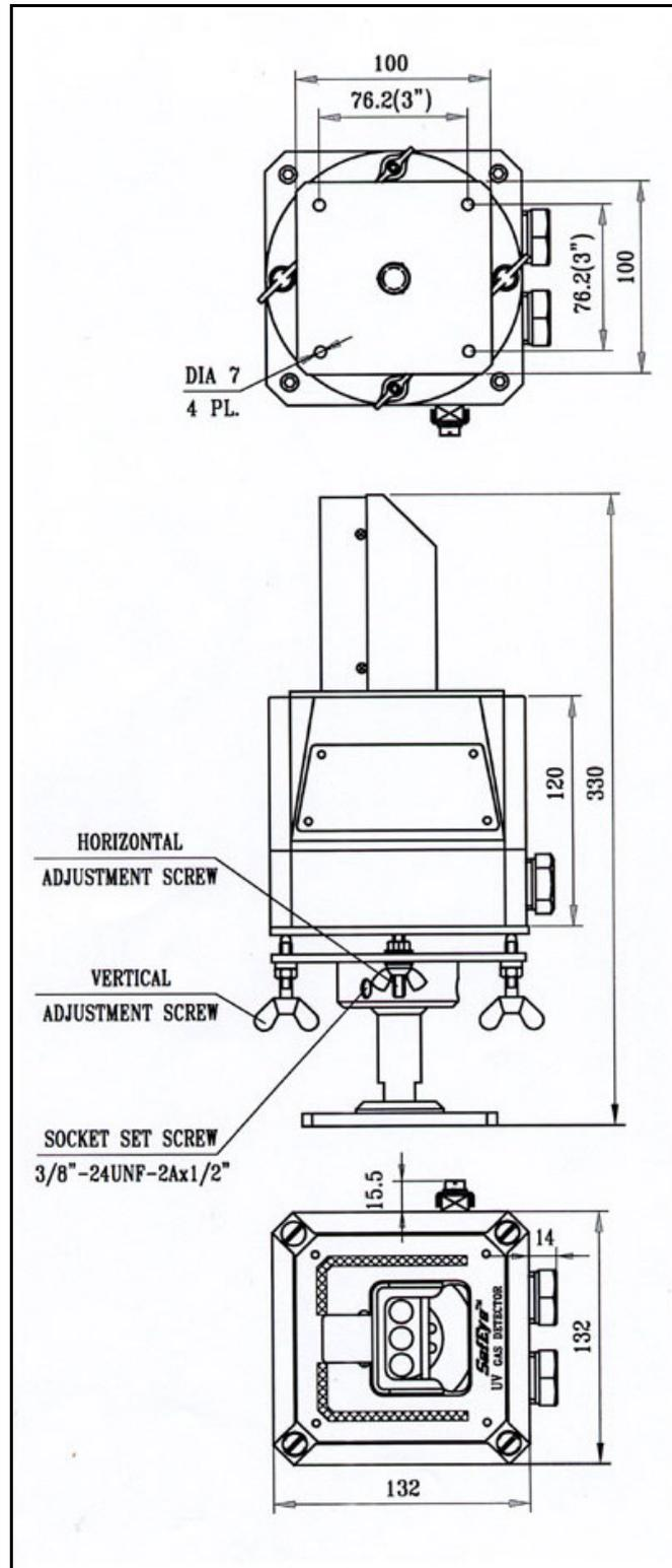
Figure 22. Detector Outline Drawing With Swivel Mount
