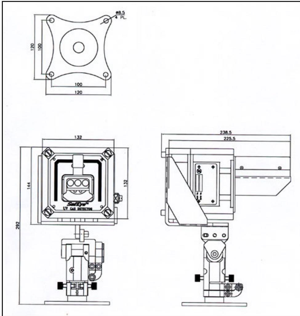
Figure 26. Detector and Tilt Mount Outline Drawing
