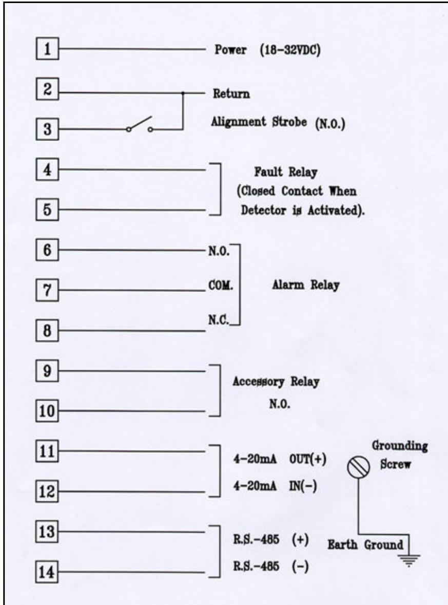
Figure 18. Detector's Wiring Diagram
