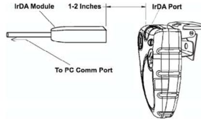
**Proper Positioning of IrDA Module**
