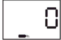
The bump test due notice is designed for instruments that are processed in an IQ Express Dock. When the bump test due notice is enabled and the ToxiPro is due for a bump test, the calibration bottle icon will be displayed at the bottom of the current gas readings screen without the triangular warning symbol.
