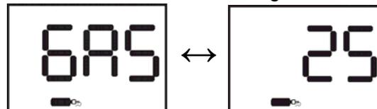
2. Apply calibration gas as shown above in figure 3.4. Once calibration gas is detected, the readout will change to show the gas reading. Note that the negated horn symbol is shown at lower left to indicate that the alarms are not operating because the instrument is in calibration mode.
