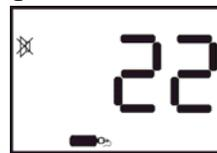
3. The calibration is fully automatic from this point on. Once the instrument successfully completes the span calibration, it will emit three short beeps and display the maximum span calibration adjustment value for two seconds.
