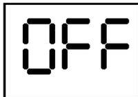
Once OFF is displayed, release the MODE button. The instrument has been successfully turned off when the display goes blank.
