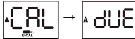
Press the MODE button to acknowledge the calibration due reminder. If the instrument shuts off when the MODE button is pressed with “cal due shown”, then the ToxiPro is configured with calibration due lockout enabled.
