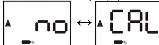
After displaying “no” and “CAL” times, the instrument will return to the current gas readings screen and the warning symbol and the calibration bottle icon will be shown, which signifies that the instrument failed the last attempt to span calibrate.
