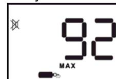
**Note: The maximum span calibration adjustment value shown is an indication of the relative health of the sensor. As a sensor loses sensitivity, the maximum adjustment level will approach the calibration gas concentration, letting you know when the sensor is losing**
