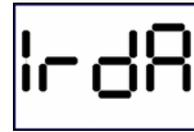
Once “IrdA” is shown release the MODE button. Then align the infrared port at the top front of the ToxiPro with the PC’s infrared port to proceed with the download. The LED/IrDA port will blink during communication with the PC. The ToxiPro should be located 1-2” (2.5-5cm) from the IrDA Port.
