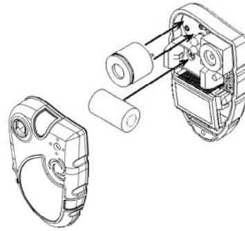
5. Install the new battery. Be sure to align the polarity of the battery in accordance with the diagram on the face of the battery compartment.
