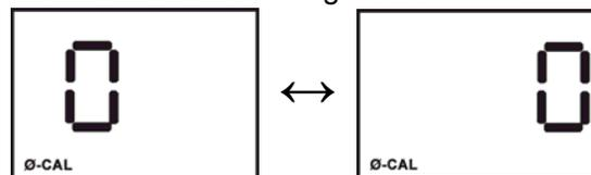
3. For instruments equipped with a toxic gas sensor, the fresh air/zero calibration is complete when the instrument begins a second 5-second countdown for the span calibration. If span calibration is not required, allow the countdown to reach 0 without pressing the MODE button. For further instructions concerning the span calibration of toxic sensor-equipped models, proceed to section 3.5.
