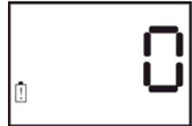
When there are less than 7 days of battery life remaining, the low battery icon will be lit.
