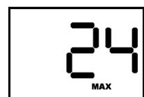
activate the backlight. Press MODE again to scroll through the screen options. Once the backlight has been lit, press MODE once more to view the MAX gas values screen. The MAX figure represents the highest gas value reading that has been recorded by the instrument during the current operating session. ToxiPro O<sub>2</sub> models will sequentially display both the highest and the lowest readings that have been recorded by the instrument in the current operating session.
