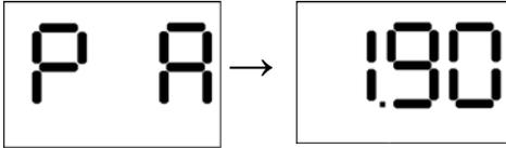
The serial number screens will then be shown: Note that the 9 digit serial number can not fit on a single screen, so it is shown on three screens. In this case, the instrument serial number is 481098190.
