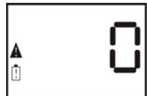
When there are less than 8 hours of battery life remaining, the triangular warning symbol on the LCD will also be shown.
