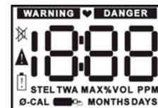
With the blank screen shown, press and hold the MODE button for 5 seconds to initiate the start-up sequence.
