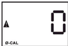
When the calibration due notice is enabled and the ToxiPro is due for fresh air calibration "0-CAL" will be displayed at the bottom of the current gas readings
