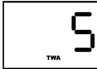
**Note: Due to the nature of the TWA calculation, the TWA value can accumulate over time and may cause the instrument to go into alarm. Honeywell Analytix recommends resetting the TWA value at the beginning of any work shift by turning off the instrument and then turning it back on again.**
