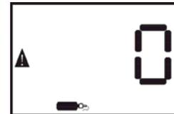
**Note:** If the Calibration Due Lockout is enabled, the ToxiPro will turn itself off following a failed calibration attempt.
