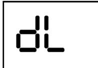
During the display of the danger alarm level, the LED visual alarm will be flashed twice and the audible danger alarm will be sounded twice. The frequency of the audible danger alarm is higher than the frequency of the audible warning alarm. The custom alarm if enabled is displayed similar to the danger alarm, but the LCD has the triangular warning symbol without the Danger or Warning symbol.
