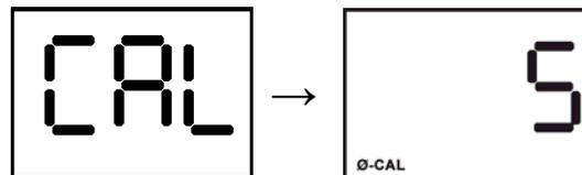
2. Press the MODE button before the end of the 5-second countdown to begin the fresh air/zero calibration. The fresh air/zero calibration has been successfully initiated when the ToxiPro alternates between the following two screens:
