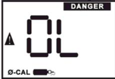
After an over range condition occurs the unit must be calibrated under controlled conditions. When an over range condition occurs, the calibration indicators are automatically activated.
