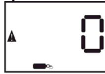
When the calibration due notice is enabled and the ToxiPro is due for span calibration the calibration bottle icon will be displayed at the bottom of the current gas readings screen along with the warning symbol.
