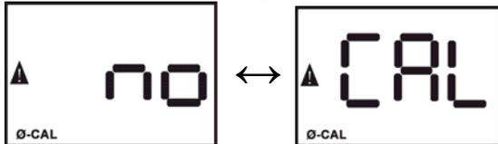
Following a fresh air/zero calibration failure, the triangular warning symbol will be lit and the “0-CAL” indicator will flash until a successful fresh air/zero calibration is performed.
