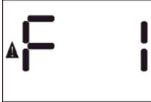
If the ToxiPro fails to detect a sensor during startup, it will show “F 1” with the caution symbol and then shut itself off. For more details, see section 2.1.
