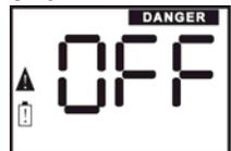
When the battery reaches a level where it can no longer power the instrument, the ToxiPro will sound a low battery alarm for two minutes while displaying the danger, caution and battery icons. Press MODE to turn the instrument off. The battery must be replaced before the instrument can be used again. If the MODE button is not pressed, the instrument will remain in alarm for as long as it can before shutting itself off.
