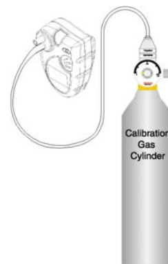
Figure 3.4 Proper bump-test/span calibration set-up for toxic sensor-equipped instruments.
