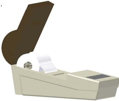
Make sure the printer is on and offer the paper into the back of the mechanism while pressing the feed switch. Keep the feed switch depressed until enough paper is fed out of the mechanism to pass through the exit slot in the lid. Feed the page through this slot and close the lid
