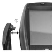
1 Remove sealing caps from the sides of the housing.
