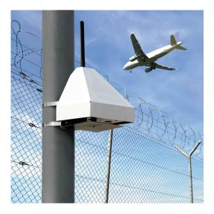
previous NO2 sensors having a massive O3 cross-gas effect (AQMesh v3.0 processing), we have made huge strides since then, particularly focusing on the key gas - NO2. AQMesh v4.0 NO2 processing reliably delivers an R2 of >0.6 in temperatures up to ~25 °C. The new v4.1 and v4.2 processing successfully tackles even higher temperature locations.
