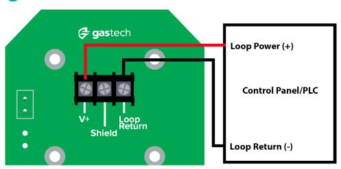
Connect the D-Guard<sup>2</sup> to a DC supply voltage of 13-28V. Make sure the outer diameter of the cable sheath is between 10 and 14 mm to allow the gland to seal properly.
