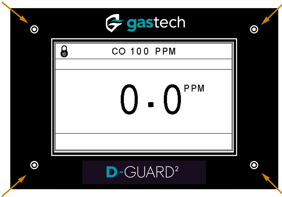
Figure 5. Arrows show magnetic sensor positions.
