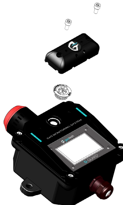
Step 2. Fit the calibration plug.
