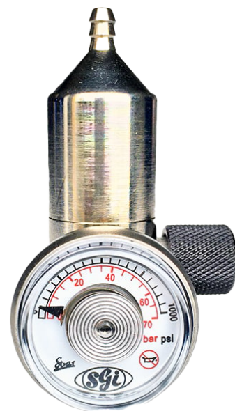
Step 4. Use a 1L / min fixed flow regulator.
