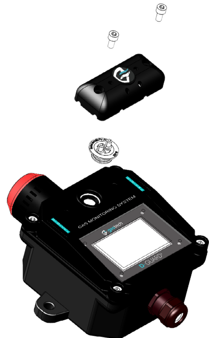
Step 2. Fit the calibration plug.
