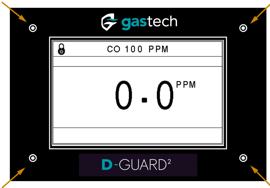
Figure 5. Arrows show magnetic sensor positions.
