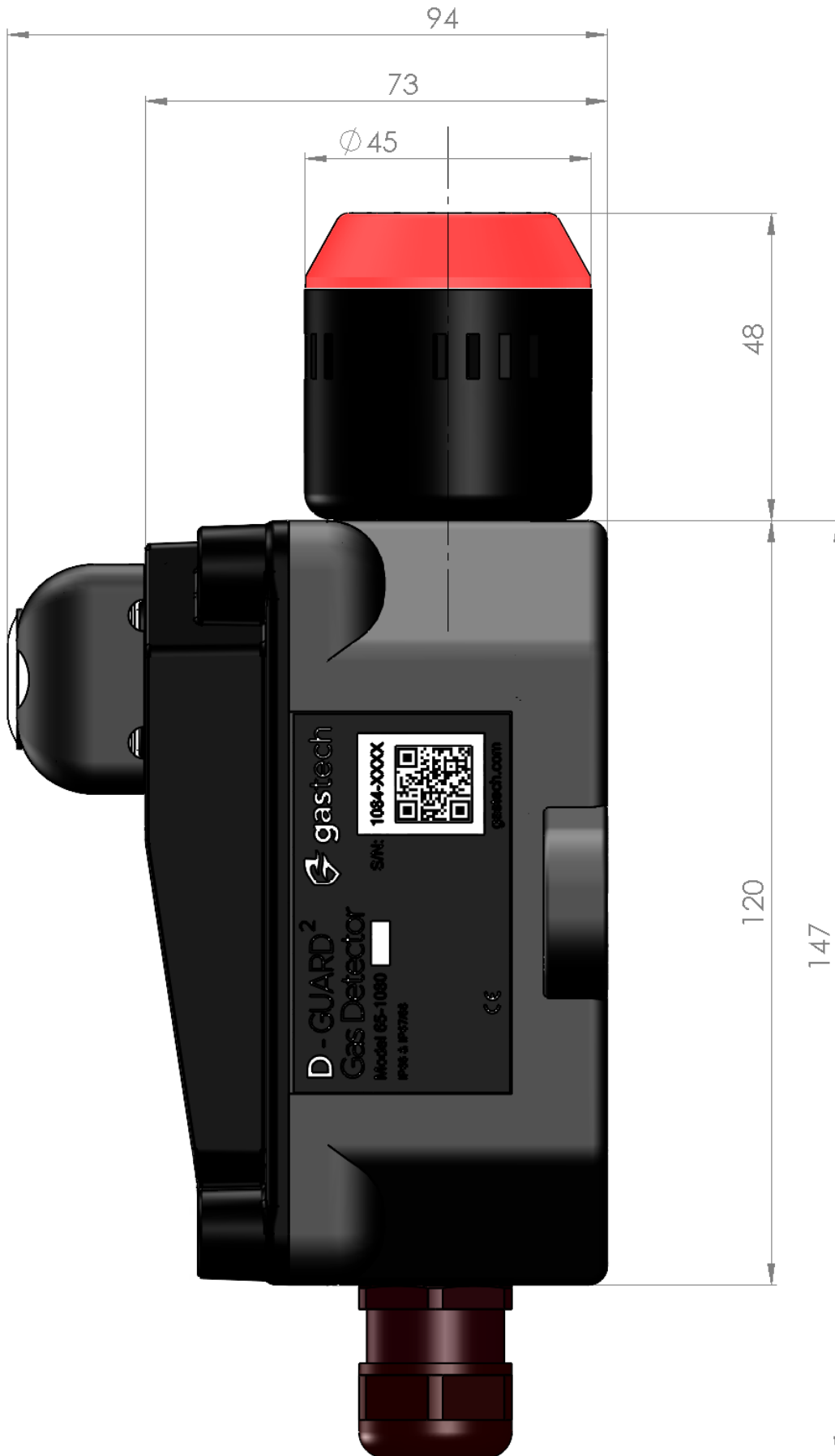
Figure 27. D-Guard 2 S dimensions in millimetres (side view).
