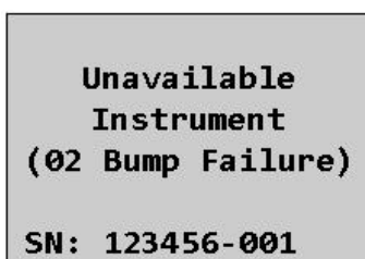
Figure 5-2. DSX-L Error Screen after O2 Sensor Failure
