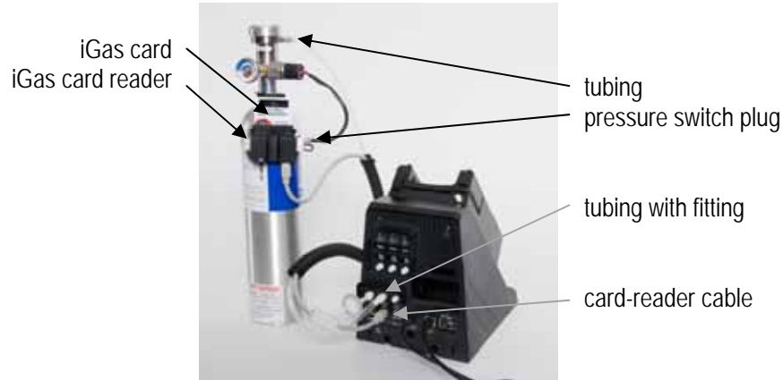
Figure 4-16. iGas Cylinder connected to DSX-L
