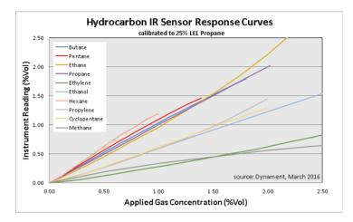
Calibrating this sensor to propane allows us to calculate the actual concentration of the hydrocarbon gases being applied using the correlations factors below.
