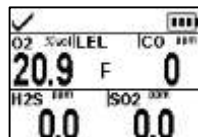
LEL sensor failure.
