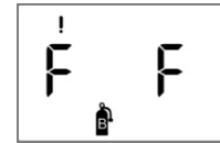
Bump test results (fail)
