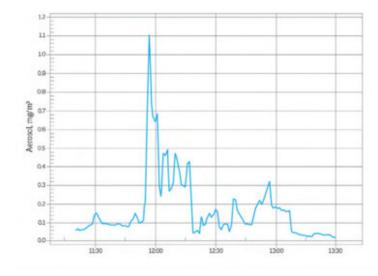
Time history - Graphically displayed, logged data can display high and low exposure concentrations that cannot be identified with traditional gravimetric sampling. This example of actual customer data illustrates the value of seeing what time peak exposure occurred. This enables an industrial hygienist to investigate the cause of the spike at 12:00 and recommend corrective actions specific to the cause without delay.
