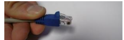
Slide boot back over lock clip
