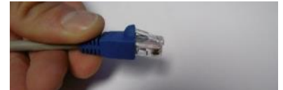
Slide boot back over lock clip
