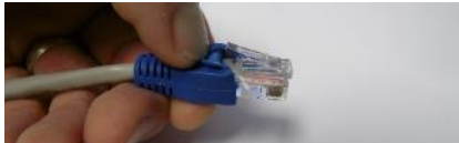
Pull boot back to access lock clip
