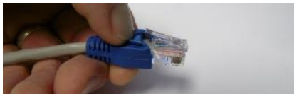
Pull boot back to access lock clip
