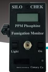
SILO•CHEK Phosphine Monitor is designed and built in Australia to detect the phosphine (PH3) levels in stored grain and horticultural products during fumigation.
