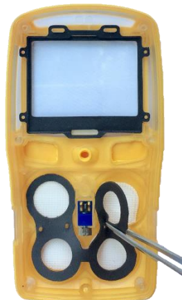
Filter & gasket replacement
