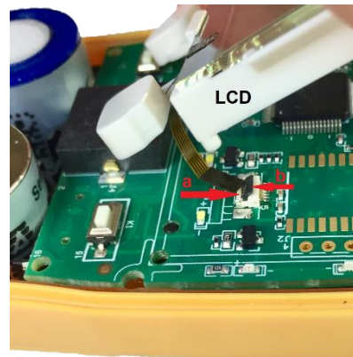
LCD connection: a. Place LCD ribbon flat onto white bracket b. Push black clamp onto ribbon to secure
