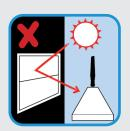
Pod clear of any surface that may reflect heat onto the pod
