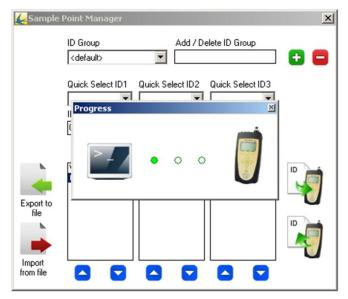
To show the progress of the data transfer taking place a "Progress" popup window will appear. The green lights moving from left right will indicate the data transfer.
