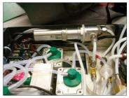
2.1.6 Route the 300mm tube coming from the bottom bulkhead through between the MEC sensors as shown, then connect to the free port of the O2 MEC flow adaptor, slightly stretching the tubing to allow for it to go over the spigot.
