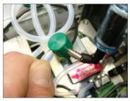
2.1.3 Remove the spare securing nuts from the bulkheads of the humidifier.
