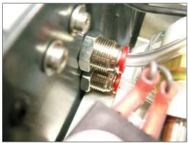
2.1.5 Route the 500mm length of tubing down to the front of the ACG+, then around and under the dewpoint sensor, connect to the outlet of the charcoal filter 6mm pushfit elbow.
