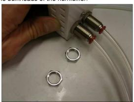
2.1.4 Take the humidifier assembly and fit the bulkheads through the two 14.5mm diameter holes as shown making sure that the bulkhead with the 500mm length of tubing fitted (Top) goes through the top hole in the enclosure base, secure in place with the provided M14 x 1mm nuts.
