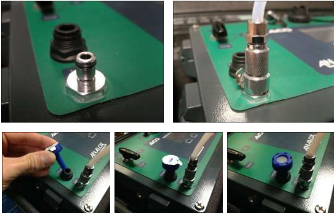
Figure 37 - A Dräger Impactor attached to the outlet port for oil mist testing
