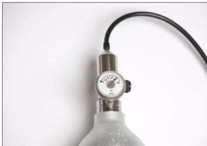
Figure 24 - Flow regulator fitted to calibration bottle
