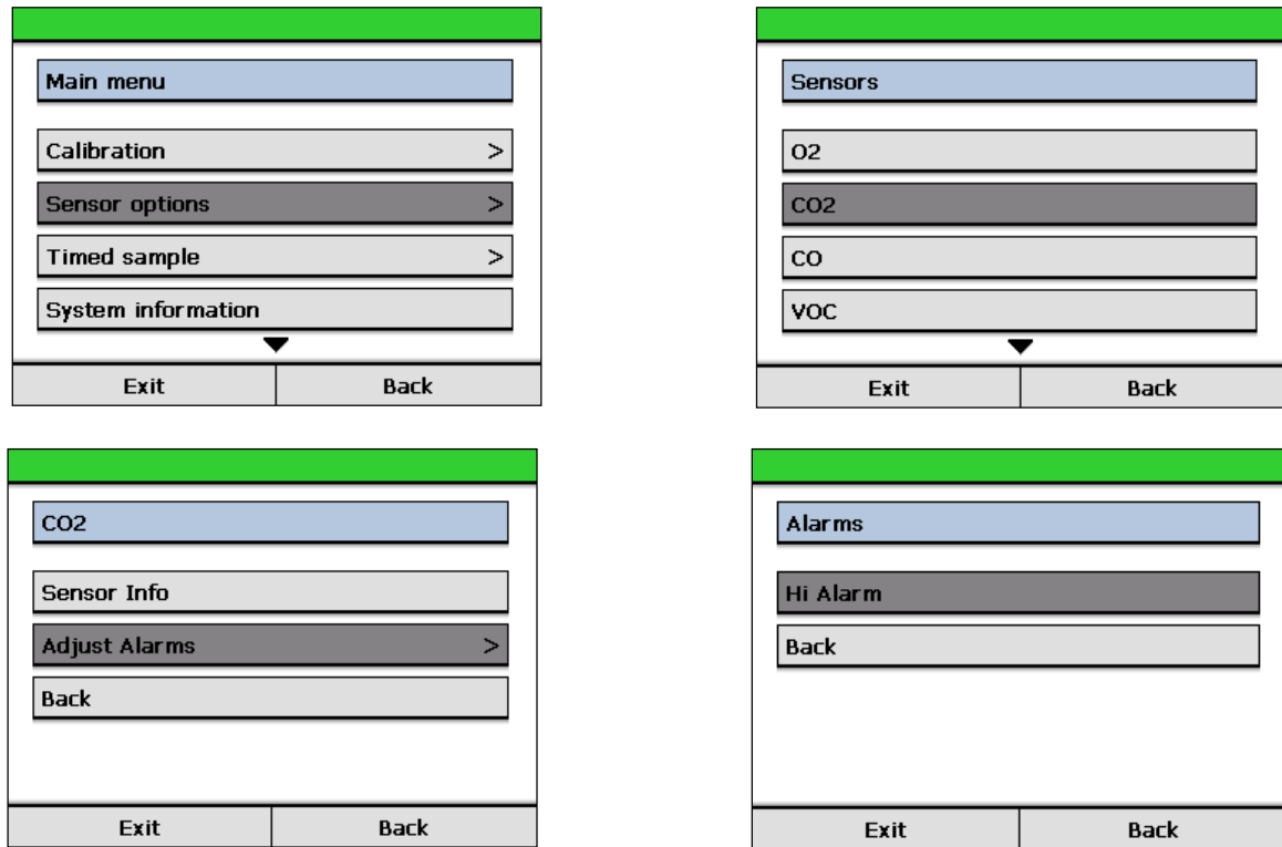
Figure 22 - Selecting a CO 2 alarm to adjust
