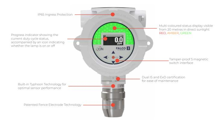
FALCO 2 11.7 features ION Science's advanced MiniPID 2 11.7 eV PID sensor, celebrated for delivering continuous precision and stability even under challenging conditions.
