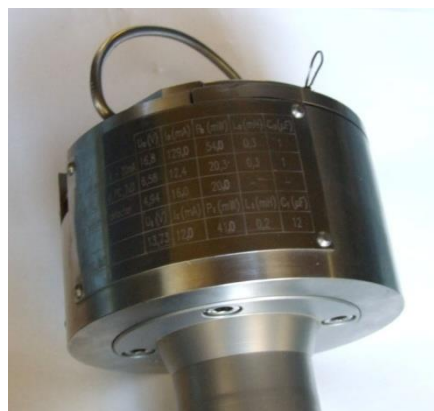
GasClam identification plates with intrinsic safety specifications.
