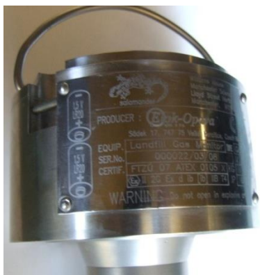
GasClam identification plates with intrinsic safety specifications.
