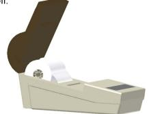
Make sure the printer is on and offer the paper into the back of the mechanism while pressing the feed switch. Keep the feed switch depressed until enough paper is fed out of the mechanism to pass through the exit slot in the lid. Feed the page, through this slot and close the lid
