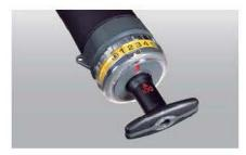
The automatic stroke counter built in the model GV-110 gas sampling pump can track up to ten pump strokes automatically so there is no chance of miscounting.
