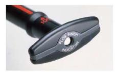
The full-stroke (100ml) and the half-stroke (SOmL) positions are marked exactly by the red line on the pump shaft, and the handle is precisely locked at those positions. The attached flow finish indicator tells you automatically when the stroke is complete. When the white disk pops out, the sample is complete.
