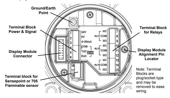
Diagram 6: Sensepoint XCD RFD Terminal module
