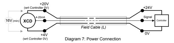
Power consumption of the detector is 5.0W. The current required to drive the detector at the minimum voltage is (I = P / V), 5 / 16 = 312.5 mA (I detector).
