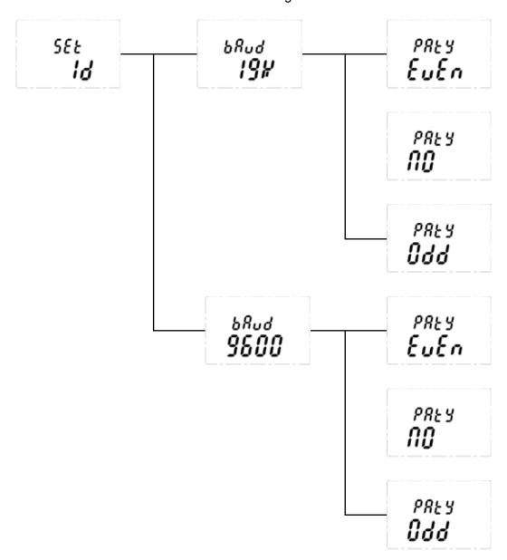
The communications baud rate and Parity Setting can also be set from this screen by using the  $^{\prime}\Delta$   $^{\prime}$  switches to navigate to the baud rate display then selecting  $^{\prime}\checkmark$ . Using the  $^{\prime}\Delta$  vswitches, highlight the proper baud rate or parity setting and select  $^{\prime}\checkmark$ . Default is Slave ID 1, 19200bps and even parity.
