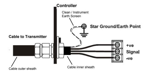
Diagram 8: Controller Grounding
