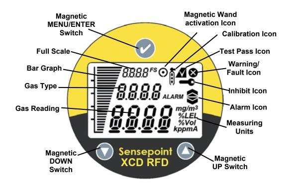
Diagram 2: Sensepoint XCD RFD Display and Magnetic Switches
