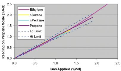
Diagram 18. Sensepoint XCD-IR (Propane) Sensor with linear cross-reference factor applied applied
