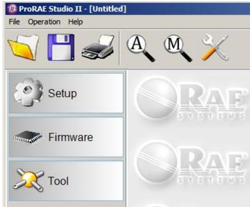
The options on the left are "Setup," "Firmware," and "Tool." Click "Firmware." This screen is shown:
