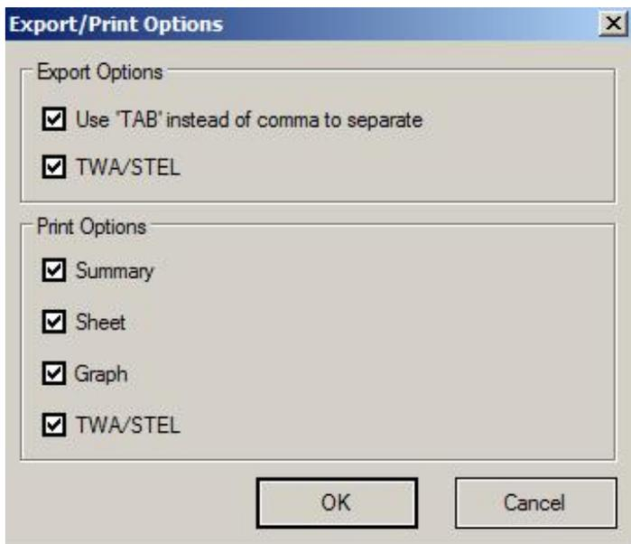
You can elect to export TWA/STEL data, and to save the data with a tab instead of a comma to separate items in each row (this is useful for files that will be imported into spreadsheets such as Microsoft Excel). In addition, there are print options, which allow you to select Summary, Sheet, Graph, and/or TWA/STEL.
