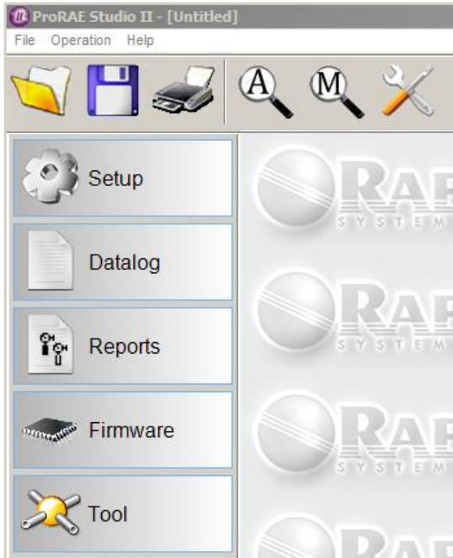
**Note:** The icons/options available depend on the operation mode and the instrument. In Data Manager mode, only Setup, Datalog, and Gas buttons are shown. In Basic User mode, only Setup and Gas are shown.
