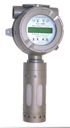
GasTech Australia Smart Guard series S-Guard™ Series GIR-3000 Carbon Dioxide CO<sub>2</sub> detector is a single source dual wavelength instrument. The sensing and reference elements are self-compensating for optical integrity and other signal inhibitors. The industry standard 4 -20 mA analog output provides remote alarm, fault and calibration signals.
