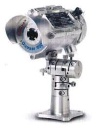
The enclosure used for both the source and detector units of, is of cylindrical construction, made of stainless steel and has two separate chambers; one flameproof and one increased safety. The equipment is shown below in a typical mounting arrangement.
