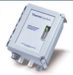
The Sample-Draw Transmitter is a single gas detector, which allows users to extract a gas sample from deep shafts, tall ceilings, wells, pits and many other locations where it is either, difficult or impossible to place a diffusion sensor. An internal motorized pump provides the power to transport gas samples to the sensor. This instrument can be configured for the detection of hydrocarbon, oxygen or other toxic gases in a wide variety of applications.
