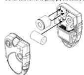
Figure 4.1: Interior view with battery and sensor removed.
